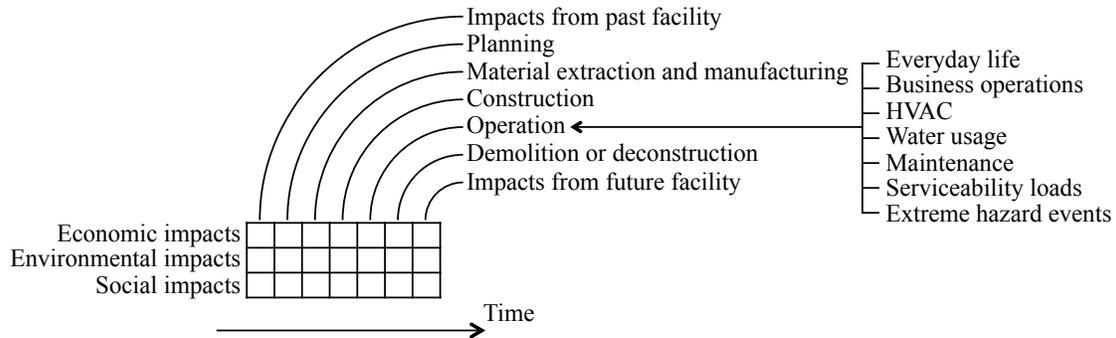
**Figure 1: Phases in the lifecycle of a building.**
