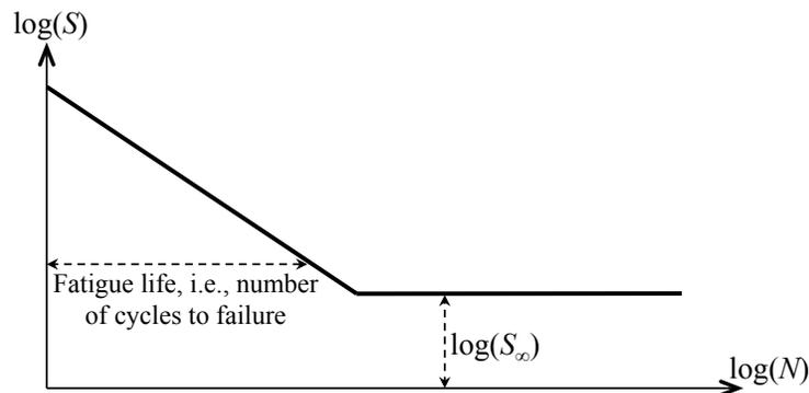
**Figure 1: Schematic S-N curve.**
