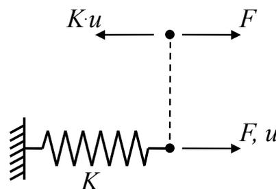
Figure 1: Simple spring with one DOF.
