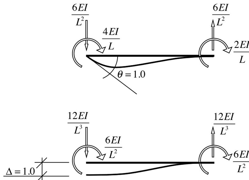
Figure 2: Stiffness values for fundamental beam cases.
