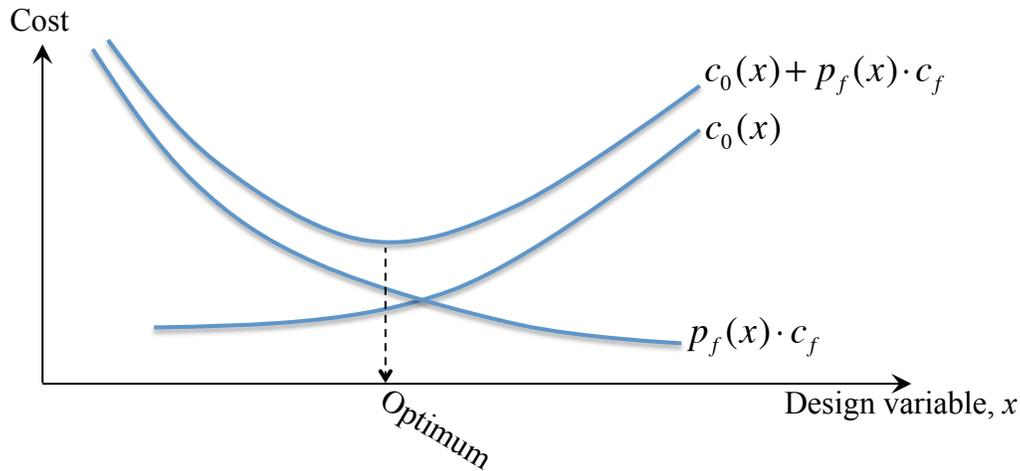
**Figure 1: Schematic illustration of reliability-based design optimization.**
